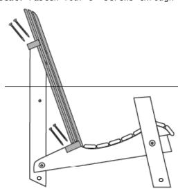
per back support and into the top of the back legs. Next, fasten four screws through the lower back support and down into the seat support.
